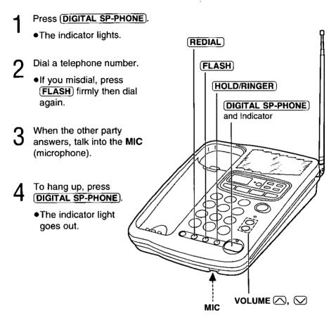
While using the speakerphone, if the handset is on the base unit, you
