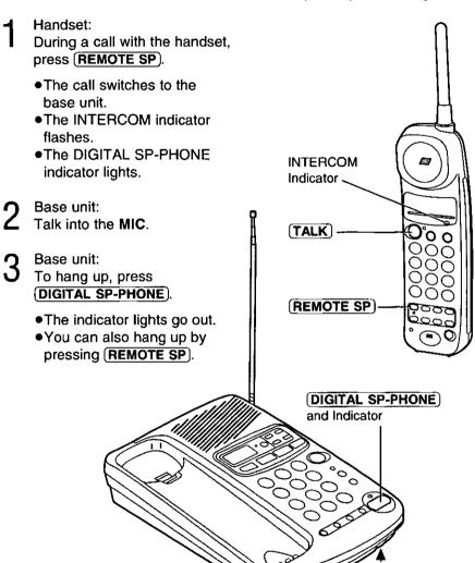
When using (REDIAL/PAUSE) or (REDIAL), dialing a stored number (p. 29), etc., press (REMOTE SP) after dialing is completed.
