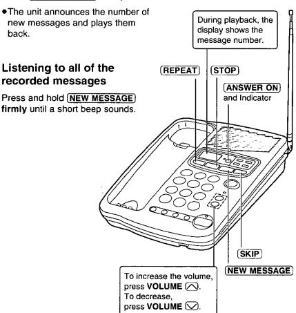
At the end of the last message, "End of final message" is heard. After the announcement, the unit will automatically turn the answering system back on.
