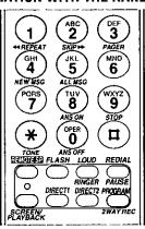
If the SCREEN/PLAYBACK indicator flashes when you press SCREEN/PLAYBACK, the answering system is off. To turn it on, press 8.
